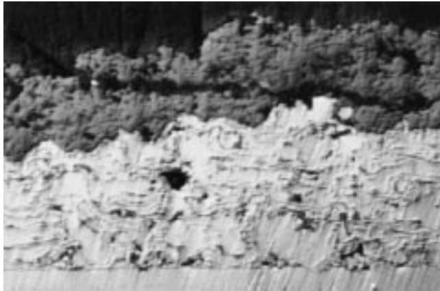
Fig. 1 Horizontal crack propagation through the bulk of the YSZ top coat. (The coating thickness is approximately 300 \mu\text{m} .)
